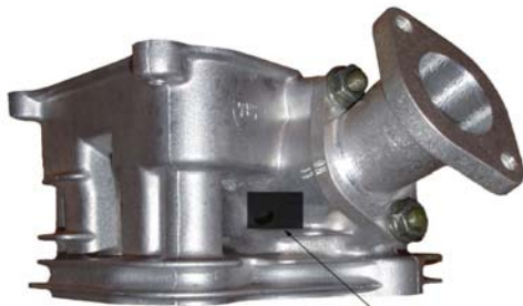
Approved Yamaha YF200 Inlet Tract Repair Area
