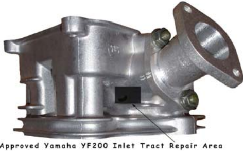
Approved Yamaha YF200 Inlet Tract Repair Area
