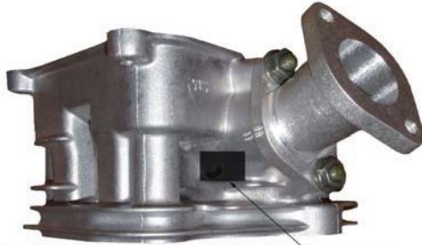
Approved Yamaha YF200 Inlet Tract Repair Area
